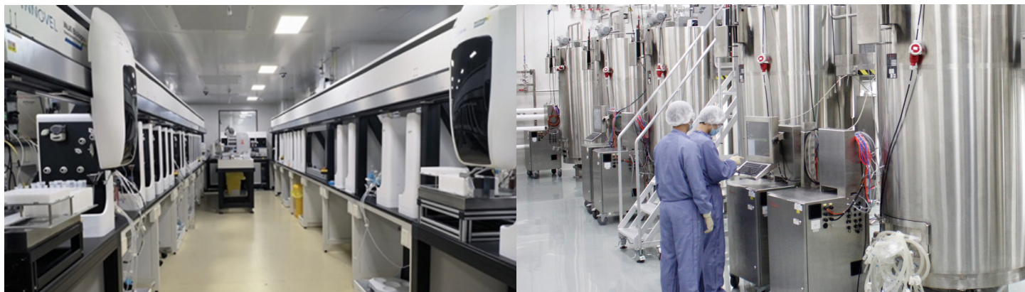
Figure 1: Automation, high-throughput (left), and disposable manufacturing (right) accelerate process development. Data from over 100 batches show that disposable manufacturing alone reduces COGS to < $80/g at a 12,000 L-scale by eliminating cleaning and sterilization steps.
